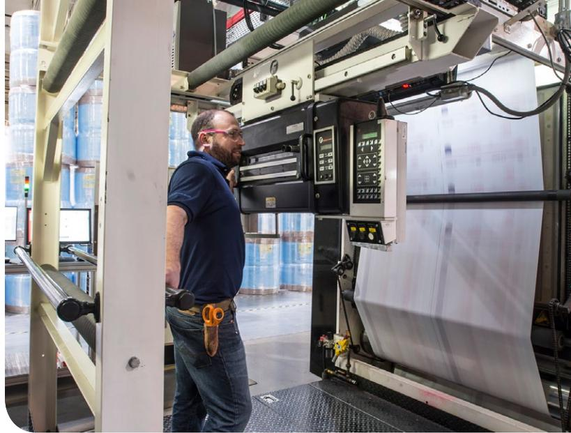
linear feet (29,870.4 meters) of material, with film slit widths ranging from about 2.8 inches (70 millimeters) to 4.1 inches (105 millimeters). We chose to use the STEP-PAC winding method, a type of traverse wind often used on fishing reels. As opposed to a parallel wind or other method, the STEP-PAC wind would allow for the least tension on the material.
