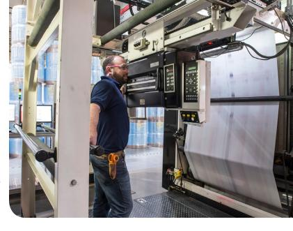
linear feet (29,870.4 meters) of material, with film slit widths ranging from about 2.8 inches (70 millimeters) to 4.1 inches (105 millimeters). We chose to use the STEP-PAC winding method, a type of traverse wind often used on fishing reels. As opposed to a parallel wind or other method, the STEP-PAC wind would allow for the least tension on the material.
