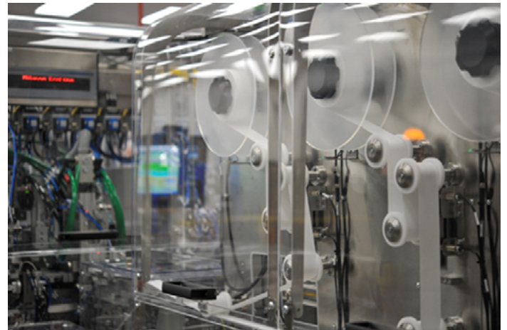
Reel-to-reel assembly and lamination of multi-layer test strips support high-speed manufacturing for large-scale medical testing programs. (Photo courtesy of Web Industries.)
