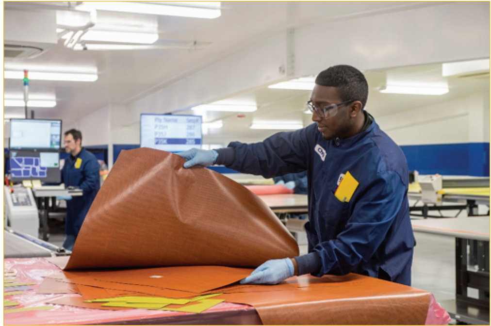
Fig. 2: Outsourcing make-ready work like ply cutting and kitting can free up valuable physical and personnel resources for aerospace fabricators
