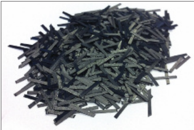
Thermoplastic chopped fibres prepared for use in compression moulding at the company's Suwanee site.
